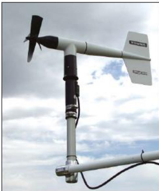
This 05106 Wind Monitor-MA is attached to a crossarm via a 17953 NU-RAIL fitting and a mounting pipe (shipped with the sensor).
