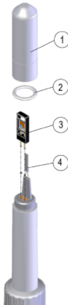
FIGURE 8-1. Changing the Filter
