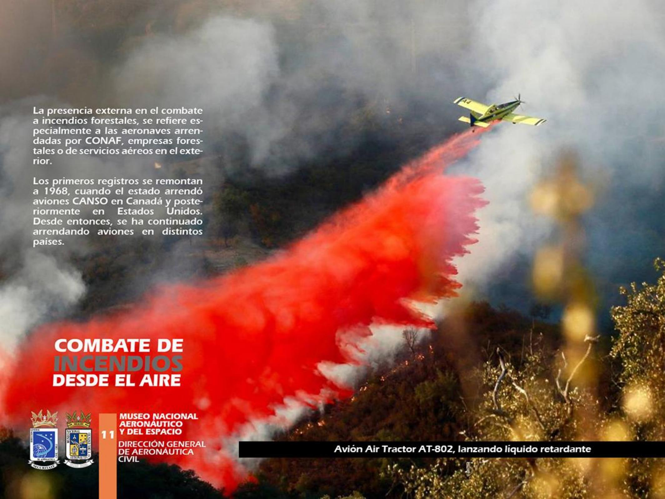
A yellow Air Tractor AT-802 aircraft is shown in flight, dropping a large volume of bright red fire retardant onto a forest fire. The fire is visible as a large, dark, smoky area on the ground, with the red retardant forming a thick, vibrant stream that falls from the plane. The background shows a dense forest with some trees in the foreground.
